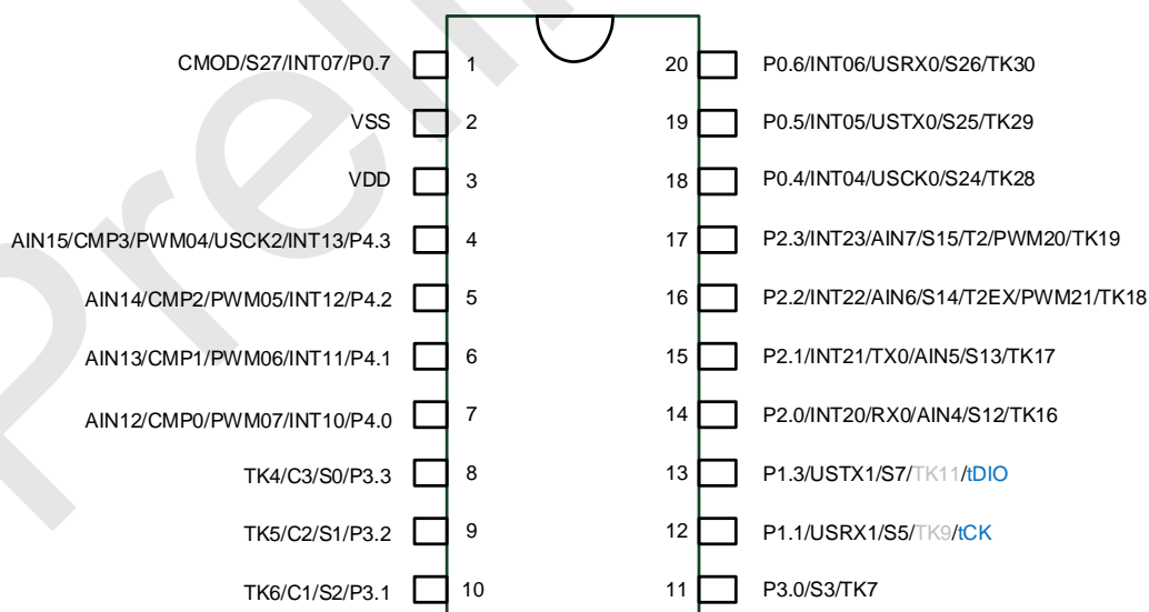
SC95F8612B Pin Diagram
