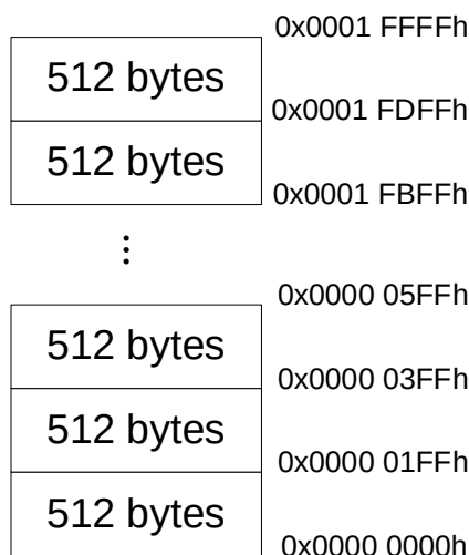
SC32F11xx7 series 128 Kbytes APROM sector partition diagram
